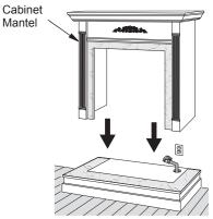
Figure 18 - Installing Cabinet Mantel
